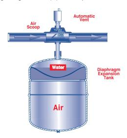
All hot water systems use expansion tanks. Older boilers typically have a steel expansion tank, which must be recharged with air periodically. Newer boilers have a pressurized tank with a diaphragm, a design that requires less maintenance.
