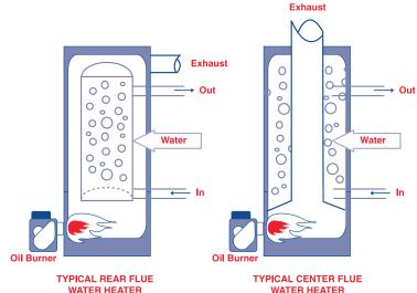
There are two direct system designs: a rear flue heater (left) in which flue gases are vented out the back, and a center flue heater (right) in which gases are vented through the top of the water heater.
