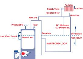
A typical configuration for a one-pipe steam heating system.
