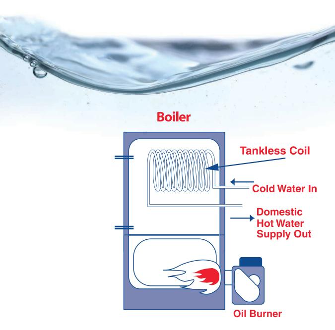
Internal tankless coil. In this type of indirect tankless water heating system, the coil containing the domestic water supply is located in the water jacket of the boiler. One drawback to this design is the absence of hot water storage; another is the need to maintain the temperature of the boiler water at a high level, high enough to heat the domestic water as it passes through the coil.
